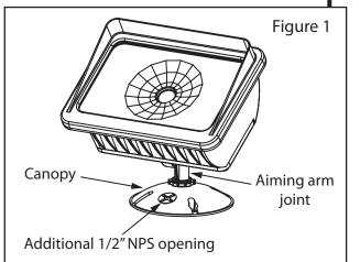
For a rain-tight seal, caulk the top and sides of the canopy and the aiming arm joint(s).
