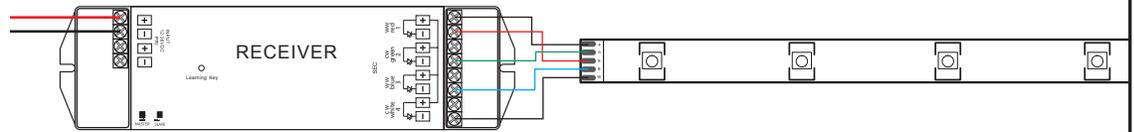
To control color, use RF-RGBW-3AAA or RF-RGBW-USB controller with REC-5A-4Z receiver (one receiver per zone); or use the Trulux RGBW application with REC-5A-4Z-WIFI (one per zone); or a DMX control with REC-DMX-5A-4Z or REC-DMX-5A-4Z-PLUS\* receiver.
