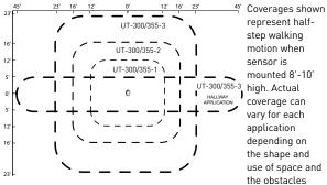
represent halfstep walking motion when sensor is mounted 8'-10' high. Actual coverage can vary for each application depending on the shape and use of space and the obstacles present.
