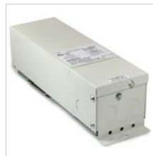
12V Dimmable Class II Hardwire Magnetic Driver with Integral Regulator for Constant Current and Voltage NMT-244/12C2D1 4x60W Voltage: 12V DC Includes: (4) 10' Power Line Connector (30' ordered separately)
