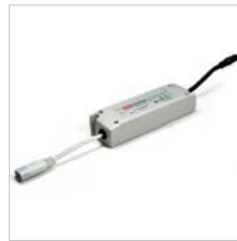
Elect. Class II Hardwired Driver NAPK-530HW/12 30W NAPK-560HW/12 60W Voltage: 12V Cable Length: 3-1/4" Input Wire: 4" Requires: NUSP-JBox for hardwire or NRA-6035 for plug in application; Power line interconnector cable to connect to Flex Light run.
