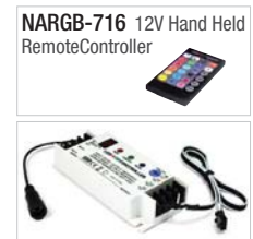
RGB Controller NARGB-716 12V Hand Held RemoteController NARGB-765 12V Controller 360W Max. A controller is required for each RGB LED Flex Light run. Installs between the driver and the power line interconnector. The controller can be used to toggle between colors or changing modes.
