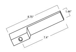
NT-326B: Black Wire Way Cover NT-326S: Silver Wire Wav Cover NT-326W: White Wire Way Cover
