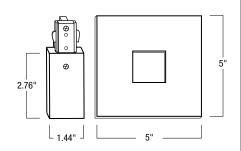
NT-311B: Black Live End Feed with Canopy NT-311S: Silver Live End Feed with Canopy NT-311W: White Live End Feed with Canopy
