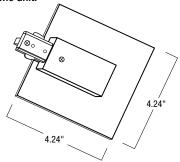
NT-352B: Black Live End Feed with Canopy NT-352S: Silver Live End Feed with Canopy NT-352W: White Live End Feed with Canopy
