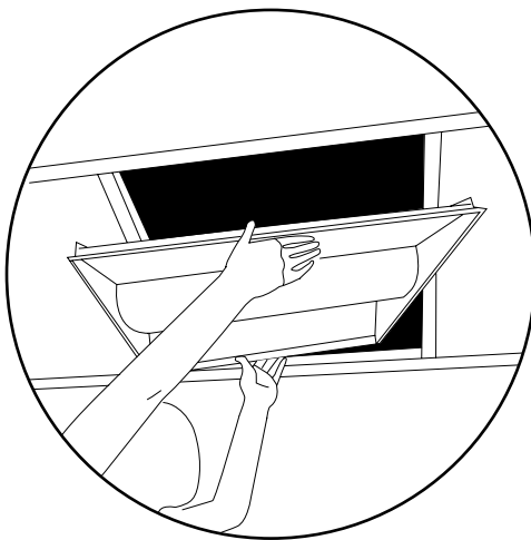
STEP 5 Install troffer into grid.
