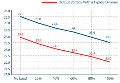
Output Voltage vs. Load
