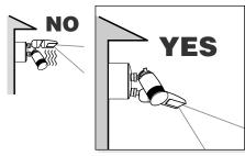
Aim motion sensor downward to limit sensing
