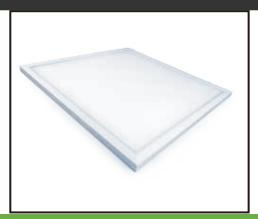
The ETi LED 42.5 Watt 4250 lumen2' x 2' flat panel LED fixture provides exceptional performance and market leading quality. Designed to mount as a drop in panel or suspension mounted, standard. The panels can also be mounted flush with an additional accessory piece. They are UL listed for use in damp and dry locations, are IC rated and are RoHS compliantwith no leador mercury. Warranty period 5 years or 60 months. Suitable for installations from -4° F to 113° F.
