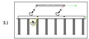
Step.3: Tighten screws on the sides of the canopy (C) to secure the fixture.
