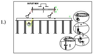
Step.1:Remove mounting bracket (A) and install to electrical box. Mark where anchors meet ceiling, remove mounting bracket from ceiling, and then drill holes using 3/16" drill bit where marked (B). Install mounting bracket and attach anchors to secure bracket at ends.
