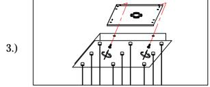
Step.3: Tighten screws on the sides of the canopy (C) to secure the fixture.
