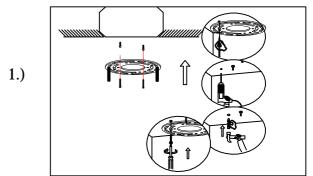
Step.1: Remove mounting bracket (A) and install to electrical box. Mark where anchors meet ceiling, remove mounting bracket from ceiling, and then drill holes using 3/16" drill bit where marked (B). Install mounting bracket and attach anchors to secure bracket at ends.
