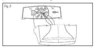
**Step 5:** Carefully tuck wires into the fixture housing (or battery box) and lift fixture onto the mounting plate. Firmly press fixture into mounting plate and, using a 3/32" hex key, tighten the 10-24 set screws until flush with housing.
