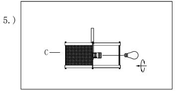
Step. 5: Install max 60 watts medium base bulb(not included) into socket.
