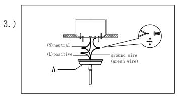
Step. 3: Wire fixture to wires in outlet box. Copper/green wire is for Ground.
