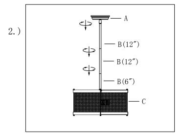
Step. 2: Run wire through stems (B) and combine stem lengths to meet desired mounting height.
