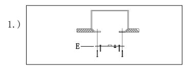
Step. 1: Install mounting bracket (E) to outlet box.
