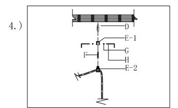
Step. 4: Install Wall plug(D) into the ceiling, And use the tapping screw(F) to lock the wire holder cap(E-1). Then install wire holder (E-2) into cap, and use wrench(F) to tighten screw(G) to lock wire holder in the cap.
