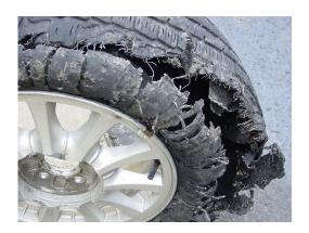
Van tire safety awareness is critical when driving 15 passenger vans. Vehicle maintenance, specifically tire inflation, has been shown to be a significant contributor in rear tire blowout. Fatal rollovers are most likely to involve tire failures. Tire blowouts can cause loss of control of a vehicle and result in these types of rollovers.
